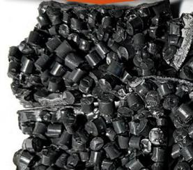
Due to the excessive temperatures, POKETONE pellets travelling down feed throat could melt and clump up. This can partially block the flow of resin into the screw and barrel and essentially run the machine out of material, while also blocking much of the flow of gas out of the machine.
