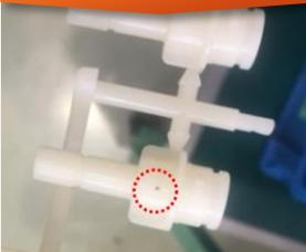
When you see black or brown specks on POKETONE molded part, most often, they are signs that the material has been degraded to a charred state, which usually means the POKETONE polymer has been at temperature for too long.
