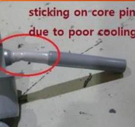
Unbalanced filling or deep core pin can cause overpacking and subsequent part sticking. With its low modulus, it could be harder to release POKETONE part than the other hard polymer part. Low mold temperature results in the mold opening before complete cooling. This causes the sticking.
