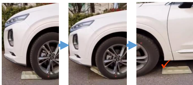
[POKETONE 聚酮餐盘 车辆加载后无裂纹或脆性断裂]
