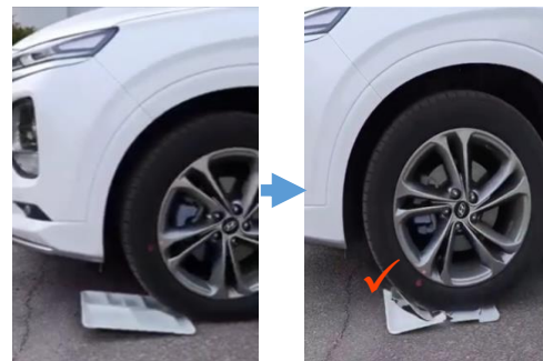
[Melamine food tray Completely Cracked after vehicle load]
