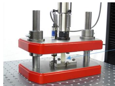
Compression Tester(ASTM D695)
