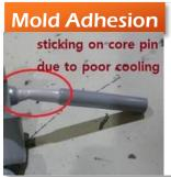
Unbalanced filling or deep core pin can cause overpacking and subsequent part sticking. With it low modulus, it could be harder to release POKETONE part than the other hard polymer part. Low mold temperature results in the mold opening before complete cooling. This causes the sticking.
