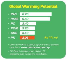
kg CO2 eq = amount of emitted CO2 per production of given resin 1kg
