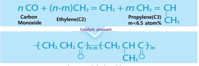
Poketone (Aliphatic Polyketone) Melting point 220°C, density 1.24g/cm<sup>3</sup>
